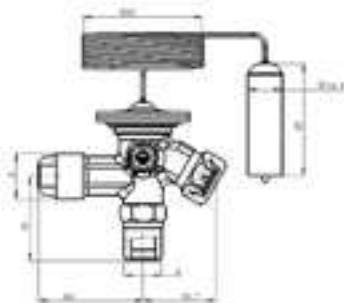
Valve Body - Connection Type: flare/flare/flare
